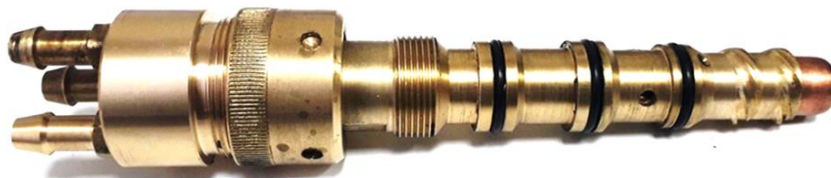
Figure 3. GVS of the PMVR-5.2 plasma torch.
