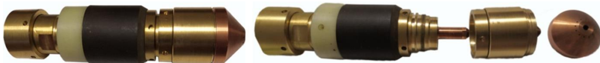
Figure 5. Experimental model of the PMVR-9.1 plasma torch (design elements).
