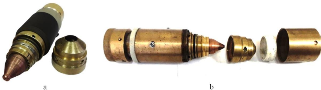
Figure 4. Experimental model of the PMVR-5.3 plasma torch (design elements).
